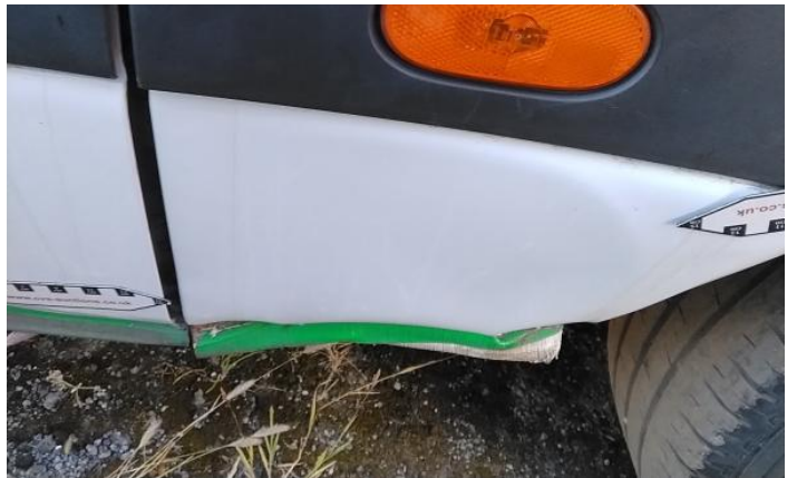
4: Sill ns Dented With Paint Damage
