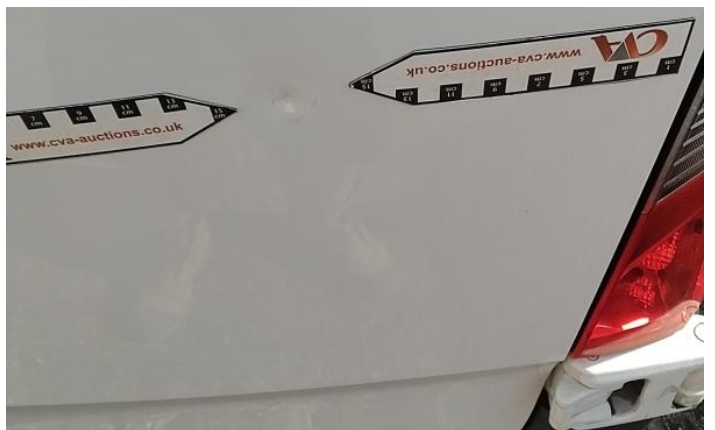
6: Qtr Panel nsr Dented Over 30mm
