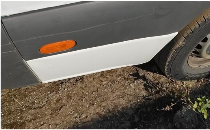
9: Qtr Panel osr Dented Over 30mm
