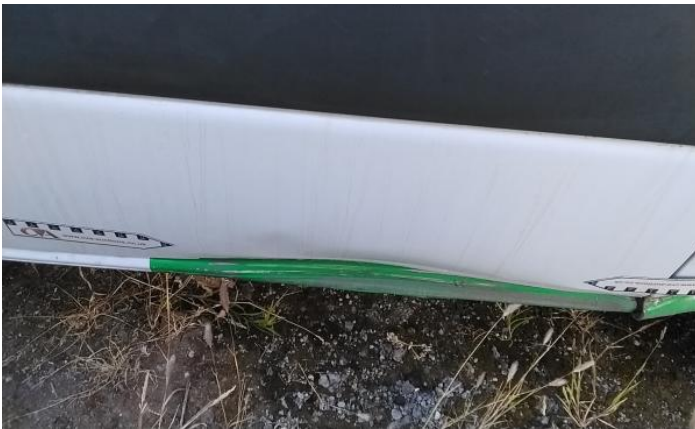
3: Qtr Panel nsr Dented Over 30mm
